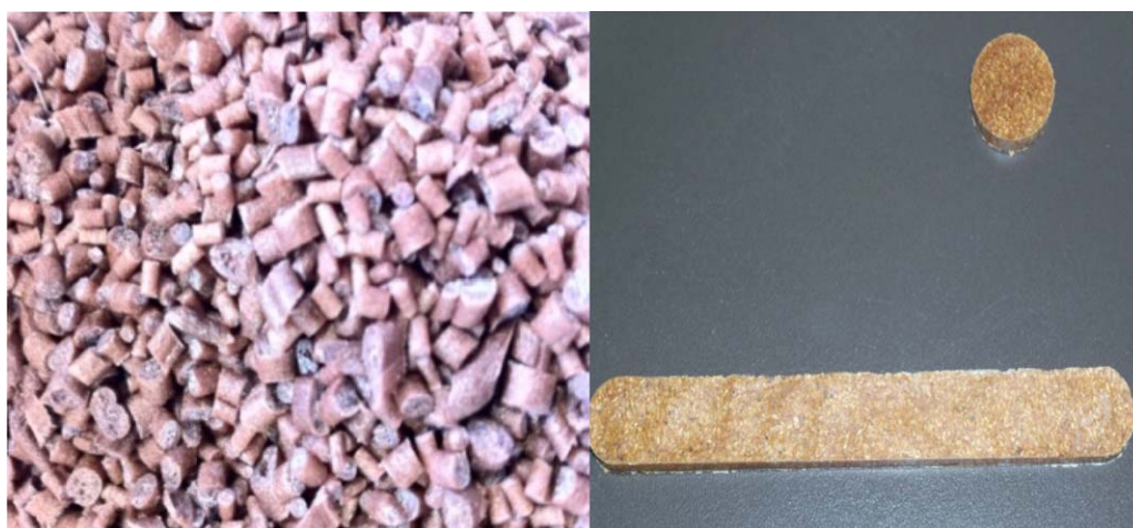
Figure 1. Pellets (left) and compression molded samples (right) of wood–polymer composites. [Color figure can be viewed in the online issue, which is available at wileyonlinelibrary.com .]
